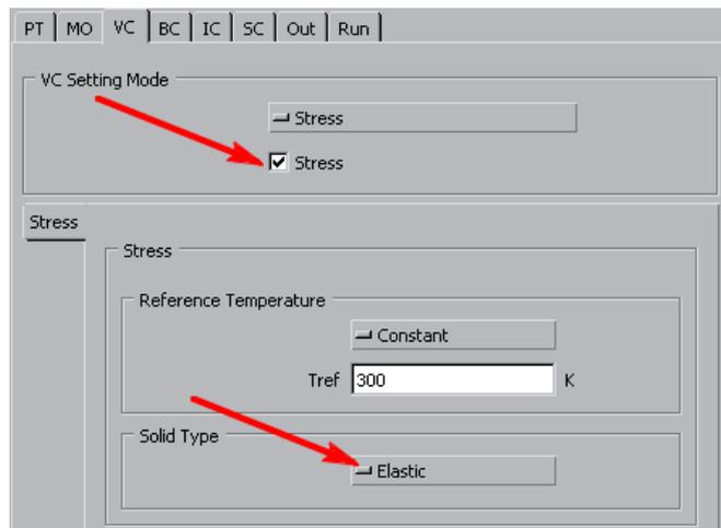
**Fig.41.** Enabling Stress calculations and deformations in volumes
