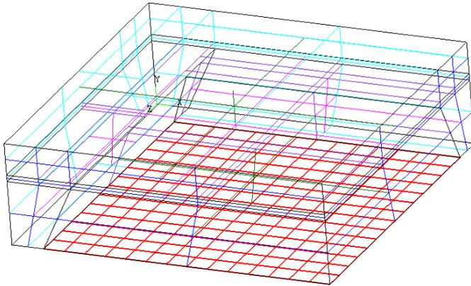
**Fig.45.** The view of the model – the contact surface between the membrane and the surroundings selected
