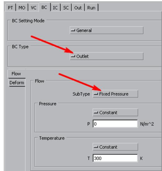
**Fig.46.** The Boundary Conditions for the gas interface
