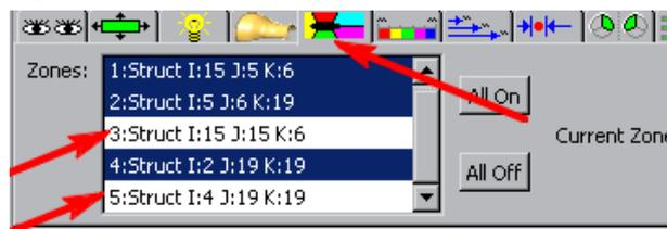
**Fig.68.** The Zone Display tab of the format area – here you can make appropriate regions of the model invisible
