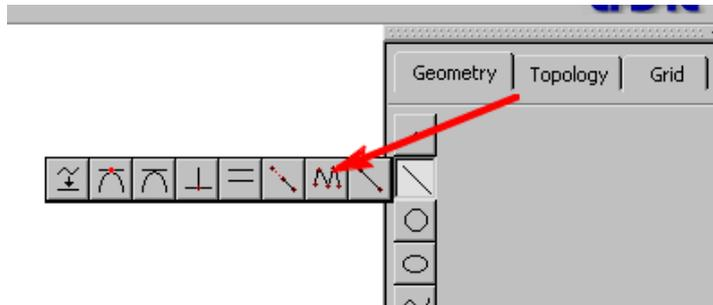
**Fig.5.** Line Creation (the Polyline function is pointed)
