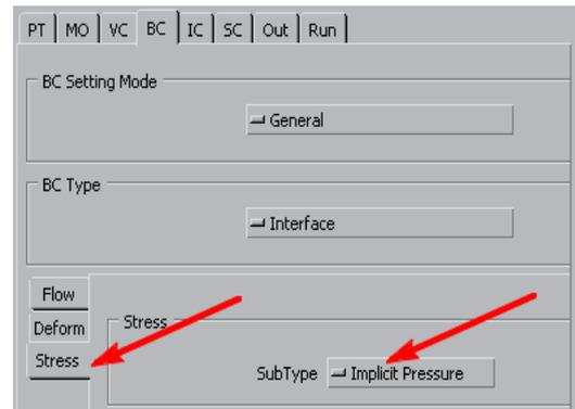
**Fig.50.** The BC settings for the top and bottom surfaces of the membrane
