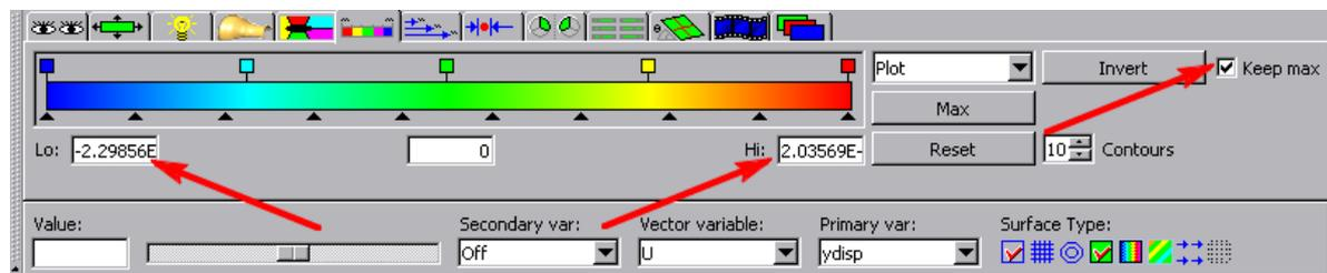
**Fig.76.** The *Keep max* option can be used to recalculate variable range
