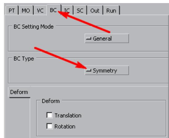
**Fig.44.** The BC tab – changing BC type from Wall to Symmetry
