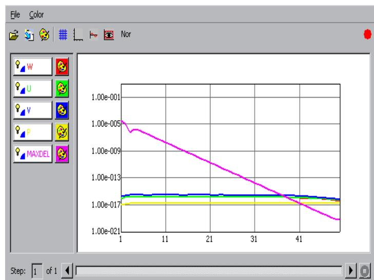
**Fig.61.** The Residual Plotter
