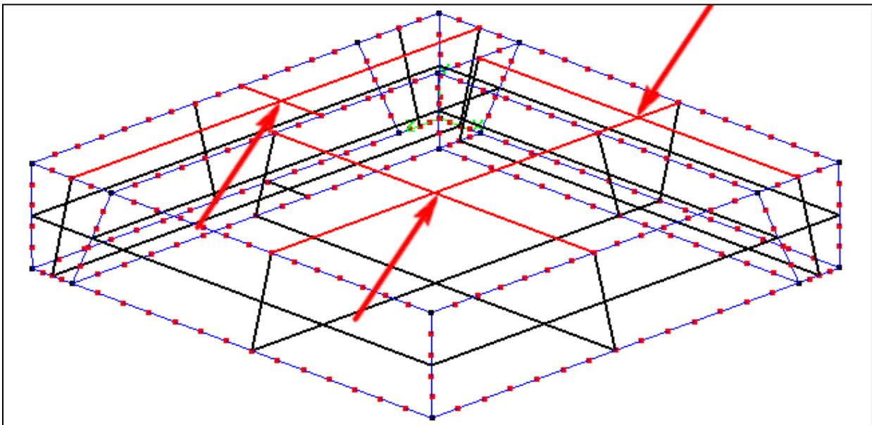
Fig.26. Before forming membrane – the handlers of the grid surfaces used to extruding marked with arrows
