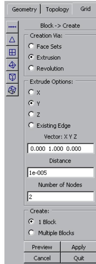
Next, select all the surface grids that form the top surface of the model (see Fig. 26). Confirm the selection with middle mouse button. In the displayed menu *Extrude Options* specify (just like in Fig. 25):
