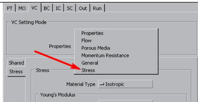
**Fig.40.** Changing the VC Setting Mode from Properties to Stress
