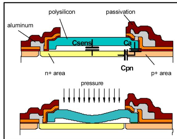
*The micro "plate capacitor" for pressure measurement*
