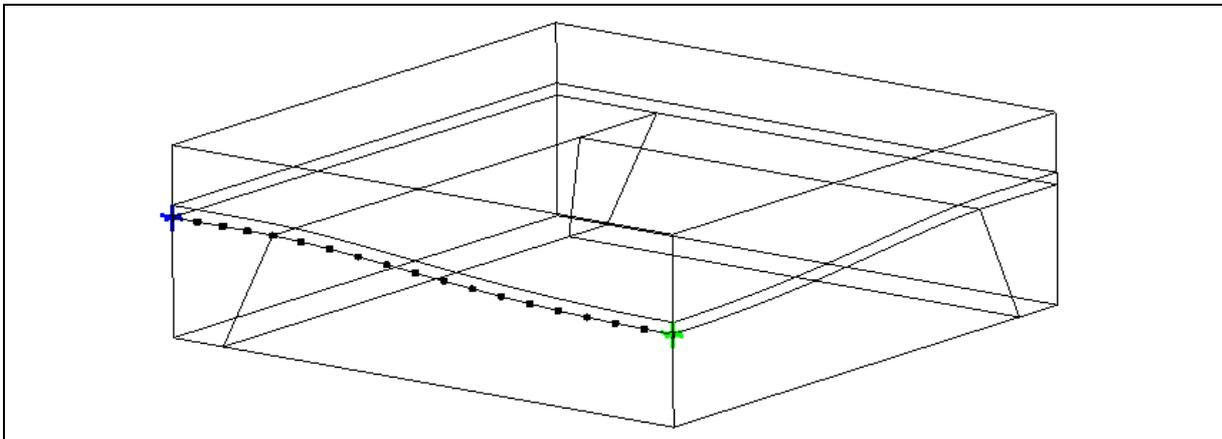
**Fig.79.** The view of the model – the probe lines should be placed along the membrane near the symmetry plane
